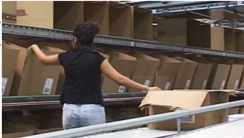
(a) Put-to-light system Lightning Pick at apparel retailer Charlotte Russe
