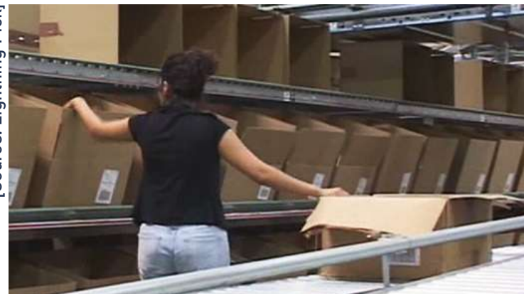
\beta_1 = \infty : Put-to-light system with many customer bins
